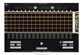
The Pattern Maker is an improved step sequencer made especially for guitar strumming. Each fret represents a quarter note and you can either add a whole chord or just a single string (if the link icon is unselected). If multiple events are in the same step, they will be strummed following our strum engine parameters.
